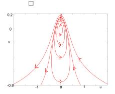
**Figure 7.** Solutions of the integrable Equation (13). The fixed point lies in the middle of limit cycles (nonlinear center). Above some threshold, solutions are no longer periodic but rather escape the vicinity of the stationary point. This illustrates the behavior of Figure 3: some canards exit to the left, while others exit to the right.
